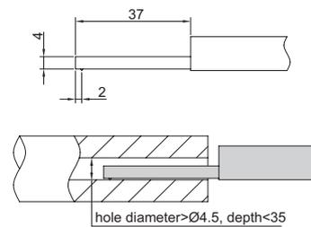
measure holes with diameter > Ø4.5mm and depth < 35mm
