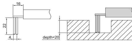
measure grooves with depth < 20mm
