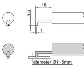
measure small rods with diameter Ø1-5mm
