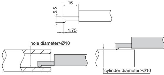
measure plane surfaces, holes and cylinders with diameter > Ø10mm
