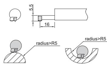
measure cylinders and holes with radius > R5mm
