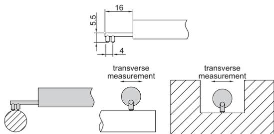
transverse measurement for plane surfaces, cylinders and grooves
