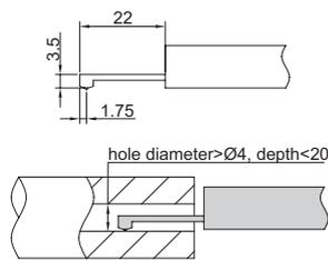
measure plane surfaces and holes with diameter > Ø4mm and depth < 20mm
