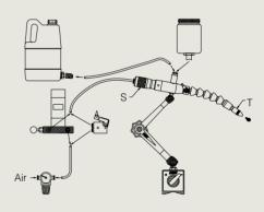
**b.** Setup for finely dispersed droplets
