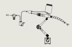
**c.** Setup to supply drops and air jet independently
