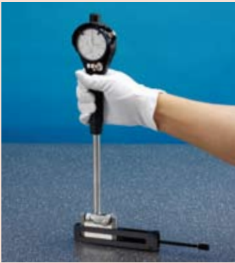
Setting a bore gage using a holder with the pair of Type I half-round jaws arranged as flat contact surfaces
