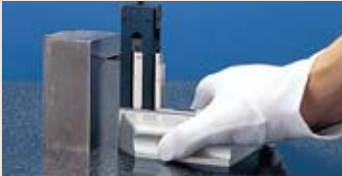
Marking a workpiece using the base, a holder and the scriber point
