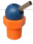
High Pressure Turret (HPT) Nozzles expand the working pressure range to a maximum 1,000 PSI, allowing a higher level of machining while providing the same LOC-LINE® quality and ease of control you've come to expect. Maximum operating temperature is 115° F.
