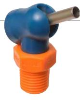
The **XR** (Extended Rotation) style nozzle features a wide nozzle swing and the ability to aim coolant below the horizontal plane, from 0 to 1000 PSI.
