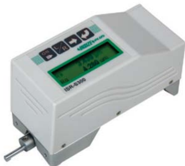
ISR-S300 (probe can't be changed)
