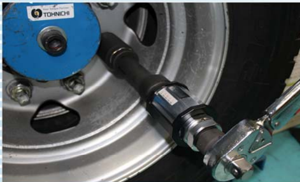
ST1000N3-G with click type torque wrench for wheel tightening
