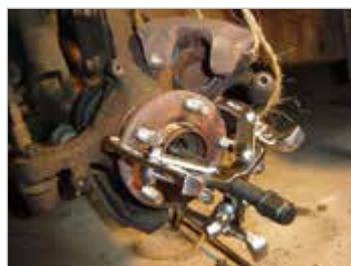
3 Jaw Puller used for removing tyre hub
