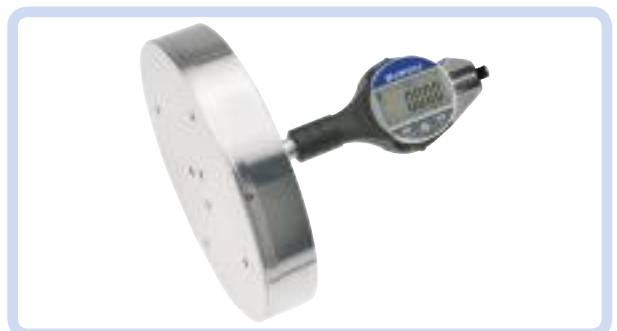
SmartPlug for large diameters (up to 280mm)
