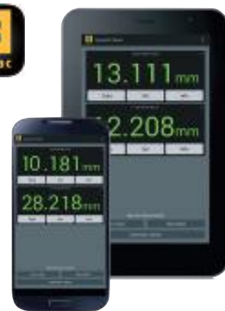
The SylvacBT Smart App allows communication with Bowers Bluetooth Smart instruments
