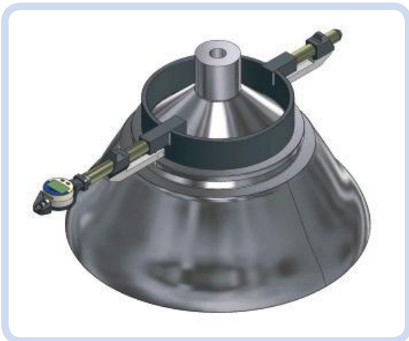
Special Universal Gauge measuring across large diameter component with central boss.
