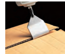
Opening strength of glued corrugated cardboard
