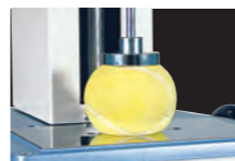
Compression test of tennis ball
