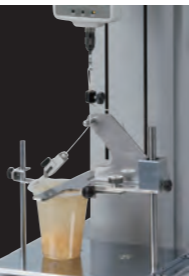
Peeling test of food container cup
