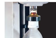
Compression test of plastic bottle
