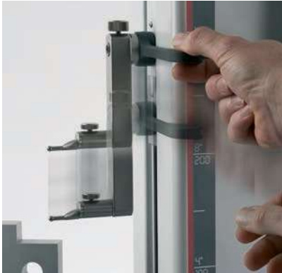
Ill. 1. Move the measuring carriage by hand in the direction of the object to be measured.
