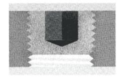
High pressure seal- Achieved through metal-to-metal contact at the large end of the plug. High load placed on the few mating threads near the top of the hole.
