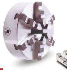
These are heavy duty self centering chucks used to grip ring type jobs with less wall thickness, the job is not damaged as gripping force is divided into 6 jaws.
