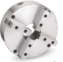
These are heavy duty self centering chucks with base hard top soft jaws. The top soft can be given required shape according to the job for better accuracy.
