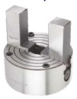
Extra blocks can be fitted on 2 no. Jaws (Extended portion is soft) required shape can be given on fixed blocks for batch work and production work.
