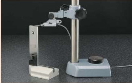
Setting a dial test indicator to a long-gauge-block stack attached to the base with a D-type connector
