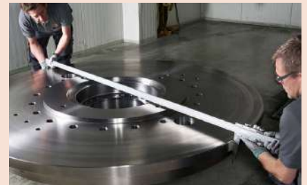
Radiused jaws for accurate ID measurement
