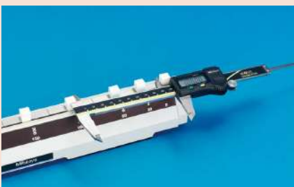
Checking accuracy of caliper (inside measurement)
