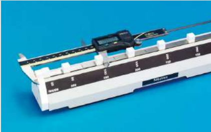
Checking accuracy of caliper (outside measurement)
