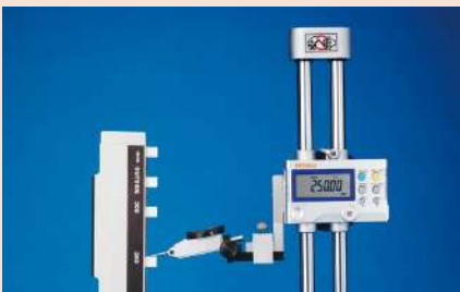
Checking accuracy of height gage
