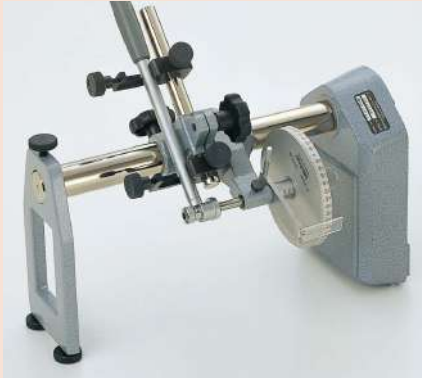
Stand for bore gage inspection (12AAK824)
