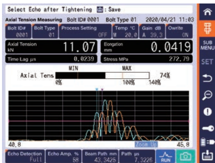
Waveform before & after giving loading
