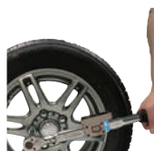
Completion of tightening process with Blue signal.
