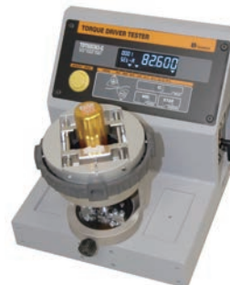
Click type RTD with TDT3-G and loading device STA.
